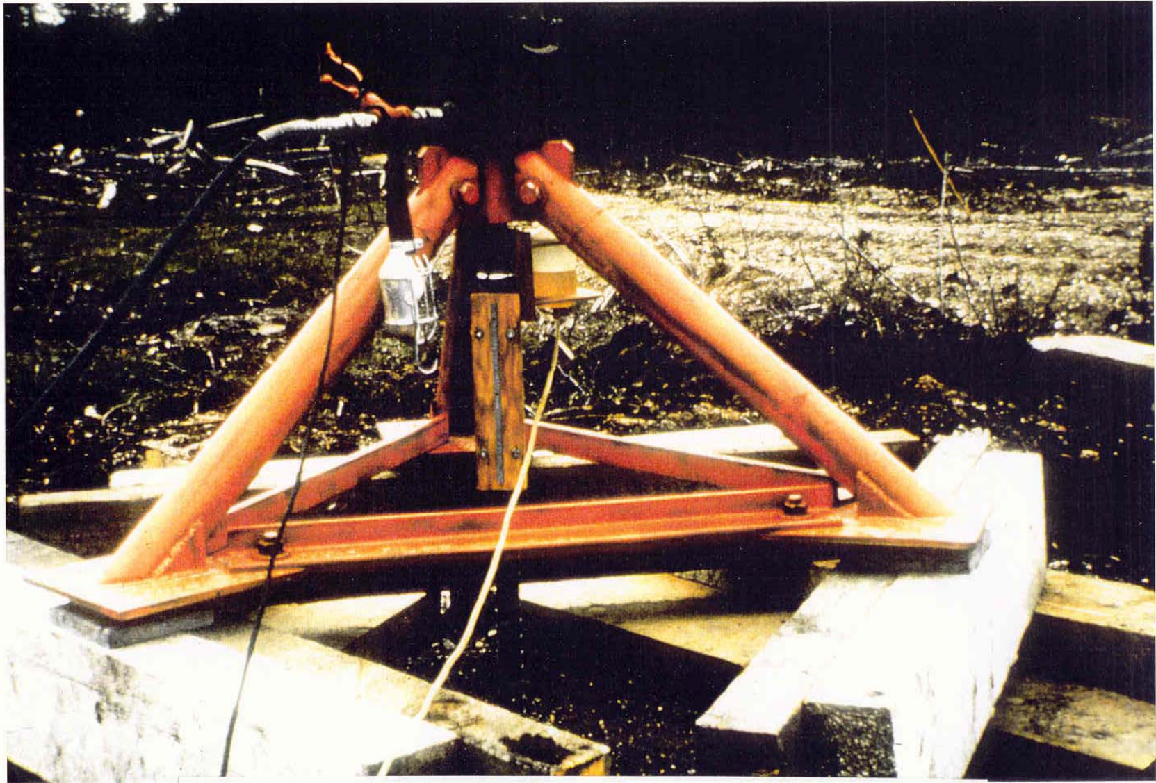
Thompson, Man. 1971. Anchor Tests in permafrost (Hank Johnston & Co.)
