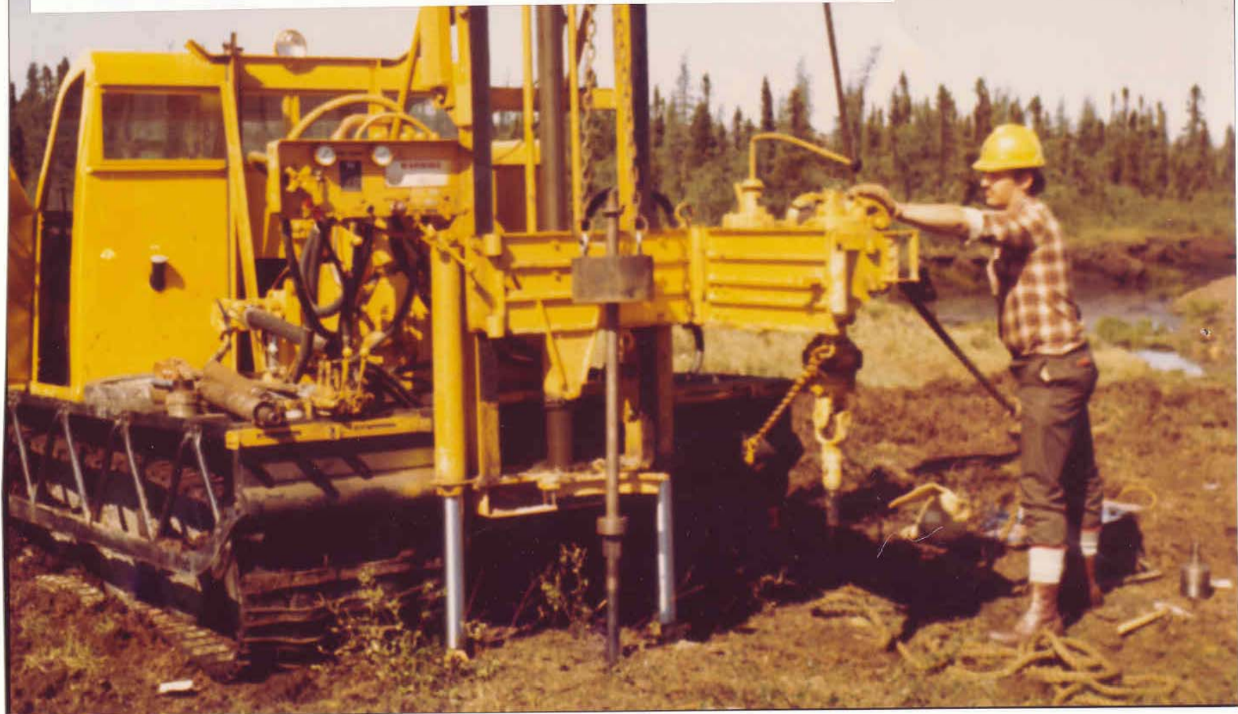
Standard penetration testing in frozen peat, Schefferville, Québec, 1972. (Ladanyi, Paquin, Gouzin, Gauvin)
