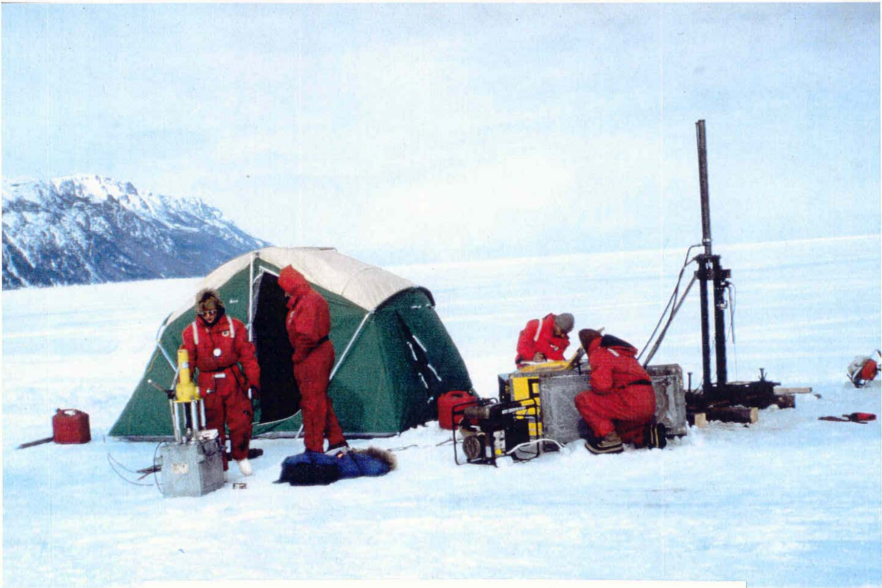
Norris Point, NF, April 1990. CPT in sea ice cover (Ladanyi, Touileb, Ducharme)
