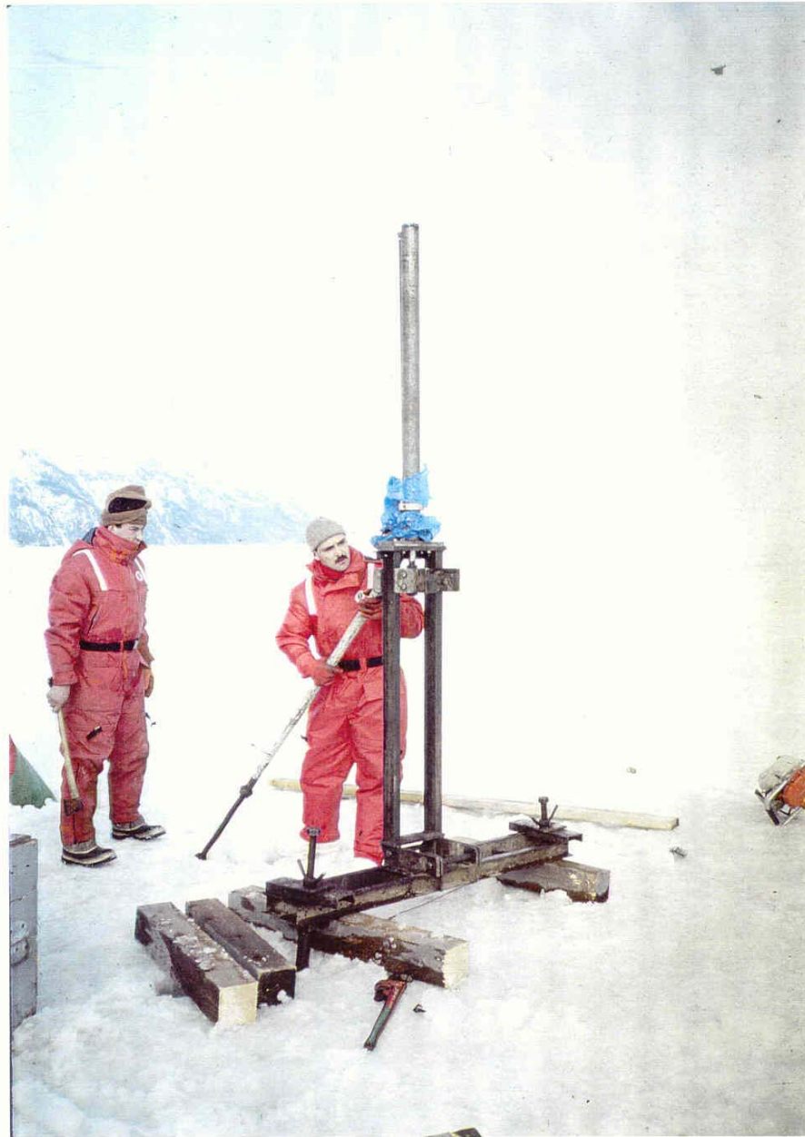
Norris Point, NF, April 1990. CPT in sea ice cover (Ladanyi, Touileb, Ducharme)
