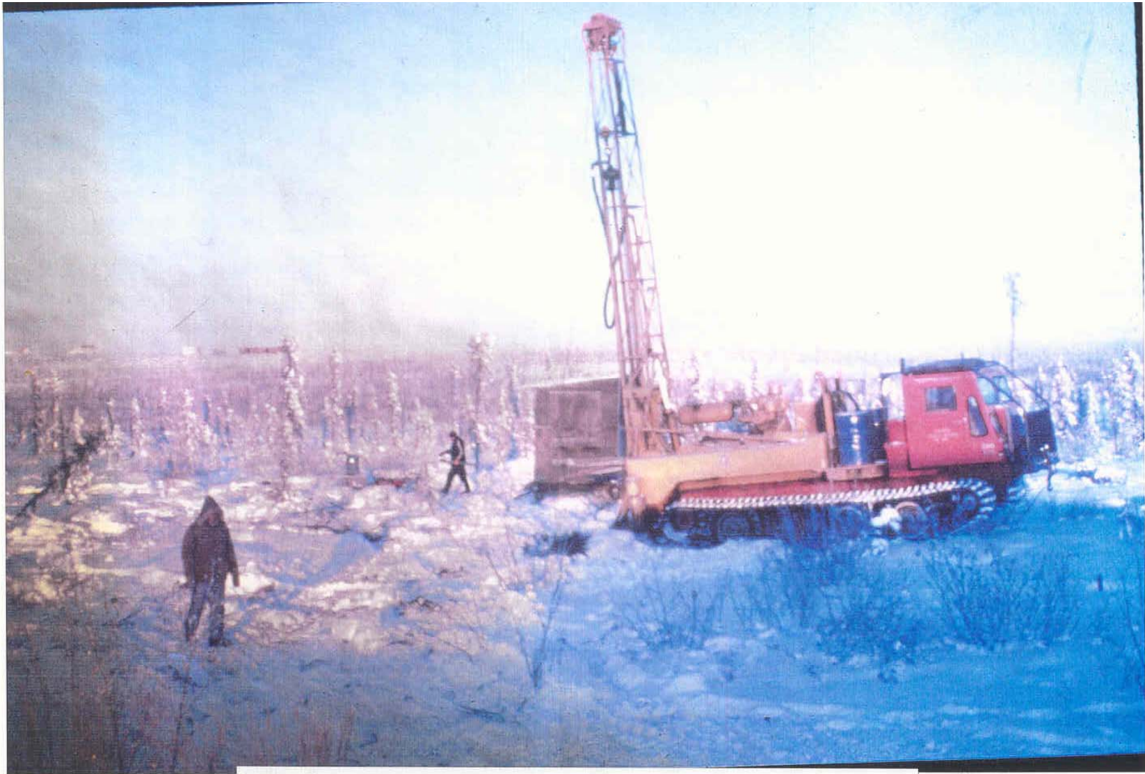
Inuvik, NWT, Nov. 1977. PMT in permafrost (Ladanyi, Barthélémy)
